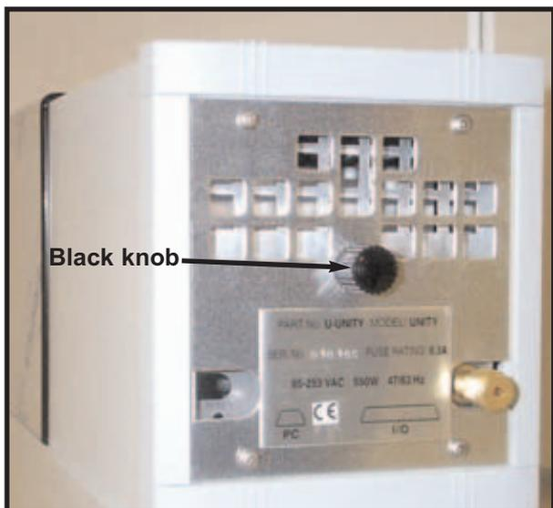
Figure 19. Photograph showing black knob fixing rear top cover to UNITY
